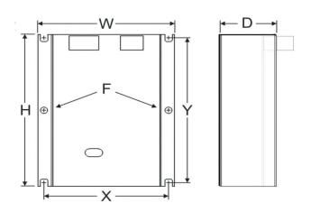
Dimensions for reference only. Use actual product for mounting template. For safe heat dissipation, mount product in orientation shown, with minimum air-gap clearance of 1.5 in. (40 mm) above and below and 1.0 in. (25 mm) at each side.
